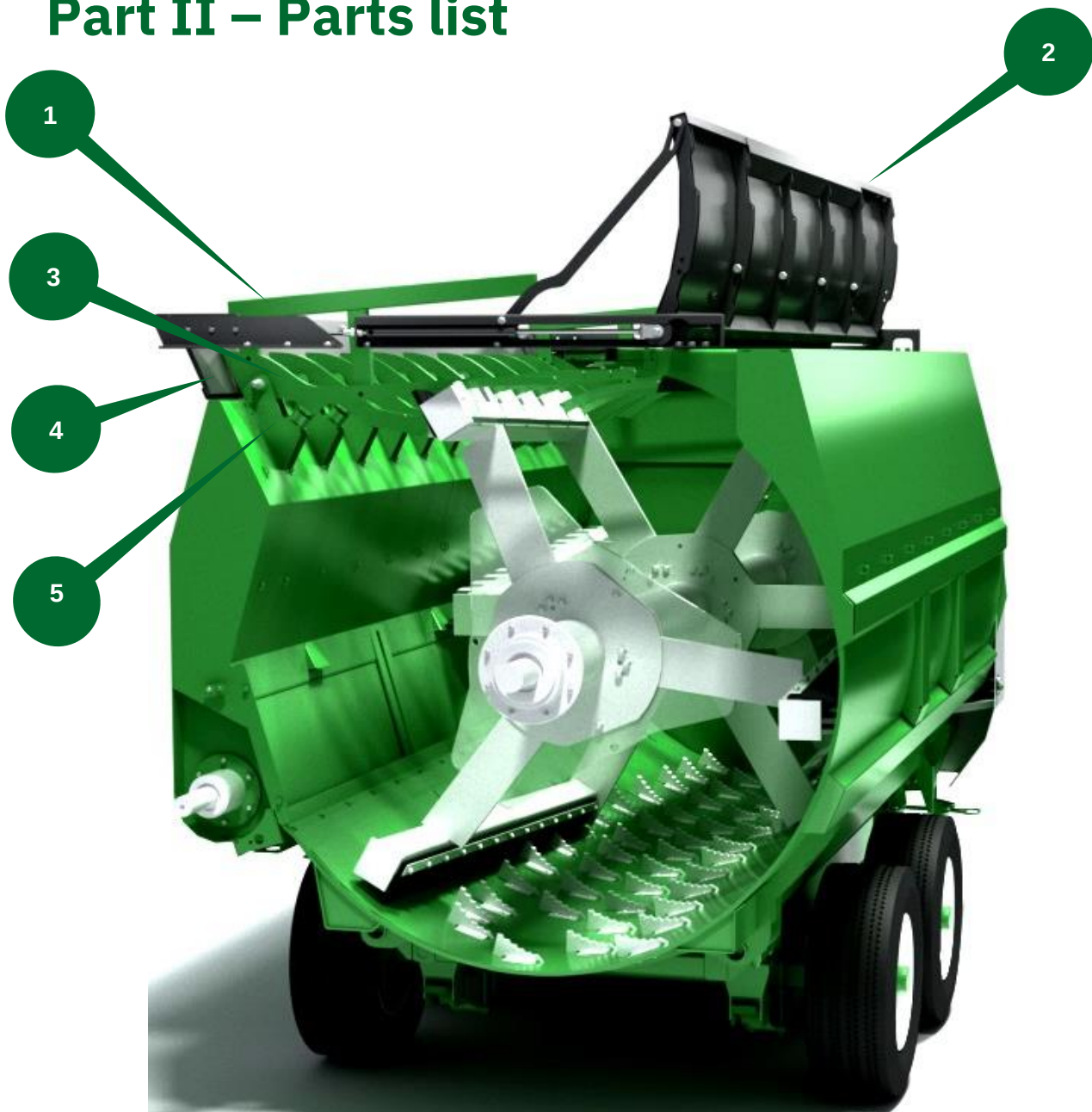
Figure 6: Bale handler general parts
